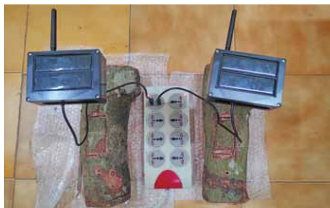
Recording of feeding sounds of CSRB grub through the acoustic device
