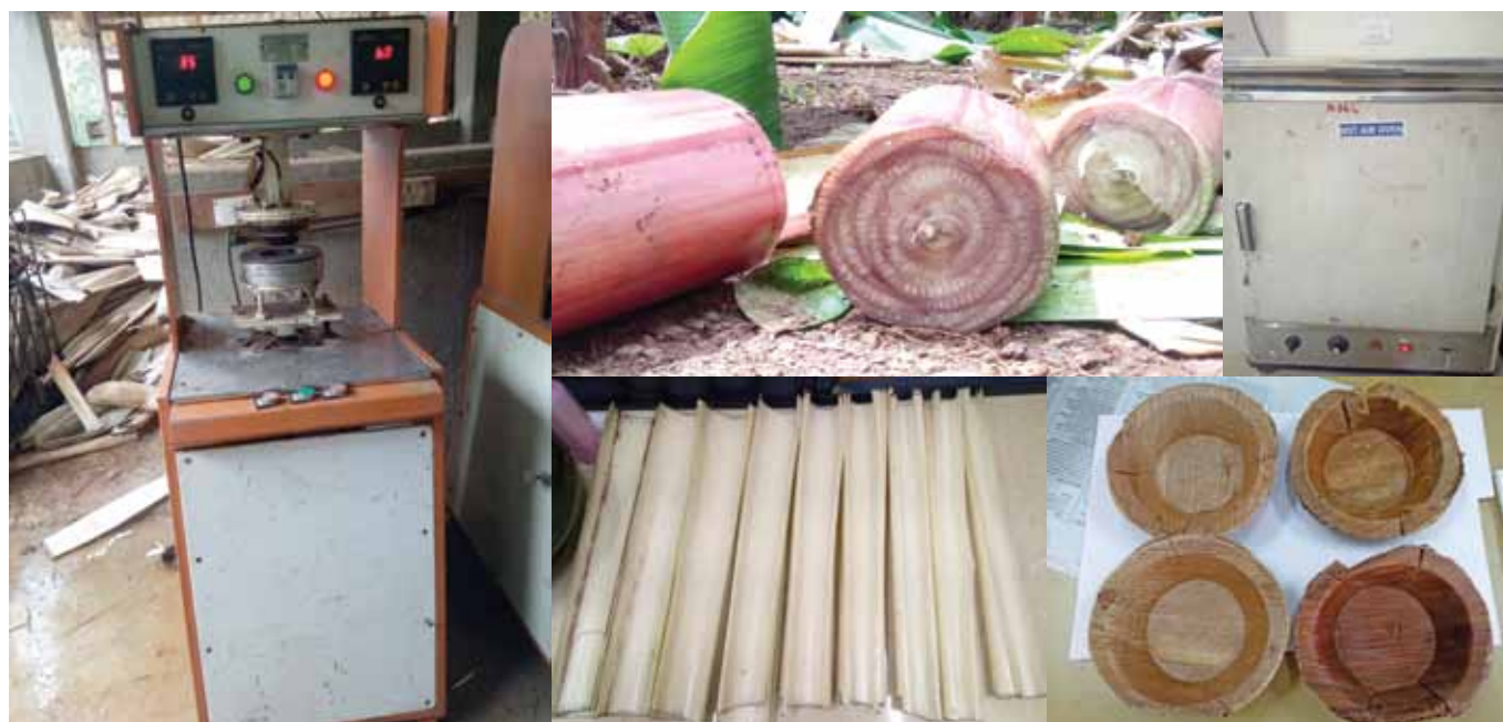
Preparation of biodegradable cups from banana pseudostem
